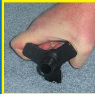
Slip the Screw Gripper over the screw head and rock the fixture left to right, snapping the head off. The screw breaks at the score that is set slightly below the wood of the floor.
